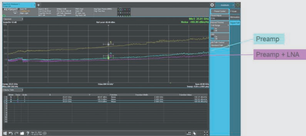
Figure 7: An example of reduced noise floor using a preamplifier and LNA, in N90442B UXA X-Series signal analyzer
